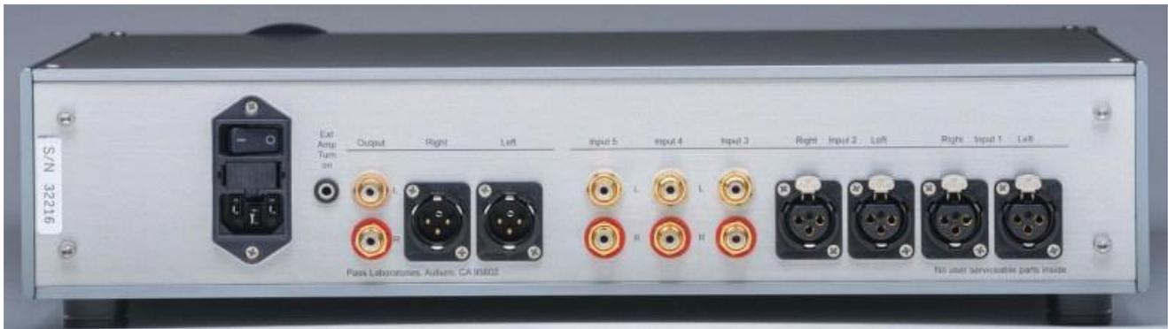
The rear panel has an IEC power cord input with a self-replaceable fuse and the main on/off switch. There are two outputs (1 x RCA and 1 x XLR) and five inputs (3 x RCA and 2 x XLR). It also comes with a very nice remote control. As the industry has come to expect from Pass Labs, the build quality is world-class and this preamp looks expensive but not overdone.
